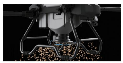
Spreader umbrella-like metal structure design, wide force area, uniform without blocking material. Bottom disc embedded in metal wheel, strength upgrade, Strong pressure resistance, more wear-resistant sowing seeds, feed, fertilizer and other operations
