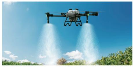
The new double centrifugal nozzle has high flow rate, good atomization and strong penetration. Strong penetration of tall plants, thick canopy of fruit trees, leaf surface and leaf back can be uniformly covered
