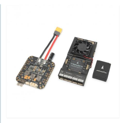
The Holybro Pixhawk RPi CM4 Baseboard combines the Pixhawk FC module with the Raspberry Pi CM4 companion computer in a compact form factor with all necessary connections for development.
