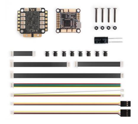
High-performance STM32 F722 MCU with speeds up to 216MHz. ICM42688P gyroscope, independent low-noise power supply. Various Ports for quick & easy setup:ESC port, Digital VTX port, Analog VTX port, Receiver port, and LED port. Built-in analog video OSD, 16 Mbytes black box,
